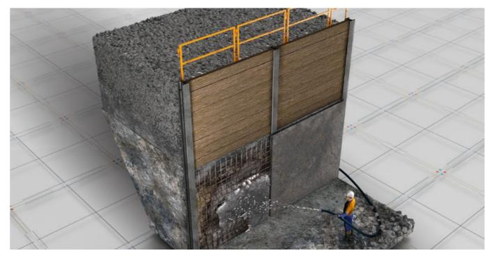
In discontinuous bored pile walls such as "king post" walls, bored piles incorporating vertical structural components (such as I-Beams, steel cages or precast elements) are installed with a greater gap. Shoring in the form of sheets, planks or shotcrete is subsequently placed between the structural elements during successive phases of the excavation process.
