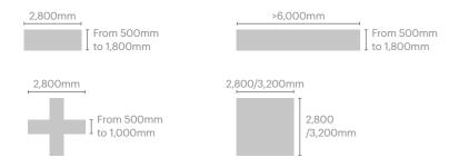
Barrettes are excavated using crane-mounted rope or hydraulic grabs, or a Hydrofraise®\*\*. In each rectangular component, typical thicknesses range between 500 and 2,400mm, and lengths between 2,200 and 3,600mm. The excavation process using rope or hydraulically operated grabs is very similar to that of LDA piles constructed under support fluid.
