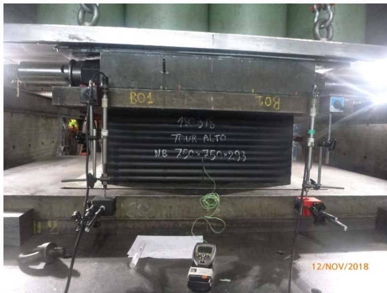
Fig. 7 – Block C pad during compression load test
